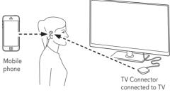
The TV Connector can be connected to any audio source such as a TV. stereo system, computer and other audio sources.
